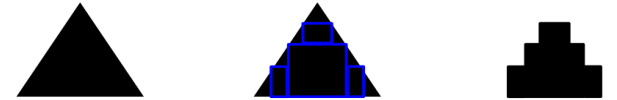
Fig. 5 Resulting Haar-like feature template when the input image is a triangle, for n = 4 .
